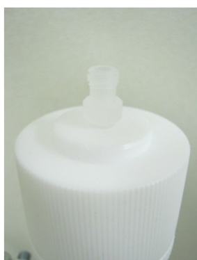
1. Injection adapter is connected to the inlet of CHIRALFLASH®.
