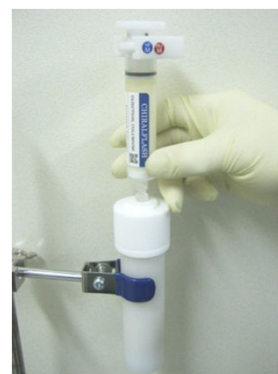
3. Fix the column adapter and the column holder to the injection column, and connect with CHIRALFLASH®.
